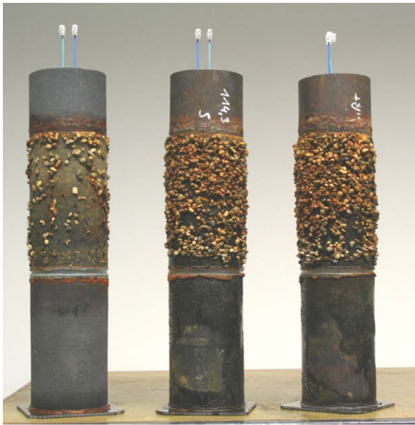
Figure 4: Picture of Samples after Testing (pre-cleaning)
