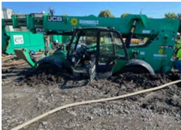
► A lull for concrete formwork is stuck after attempting to traverse an unstable Working Platform.
