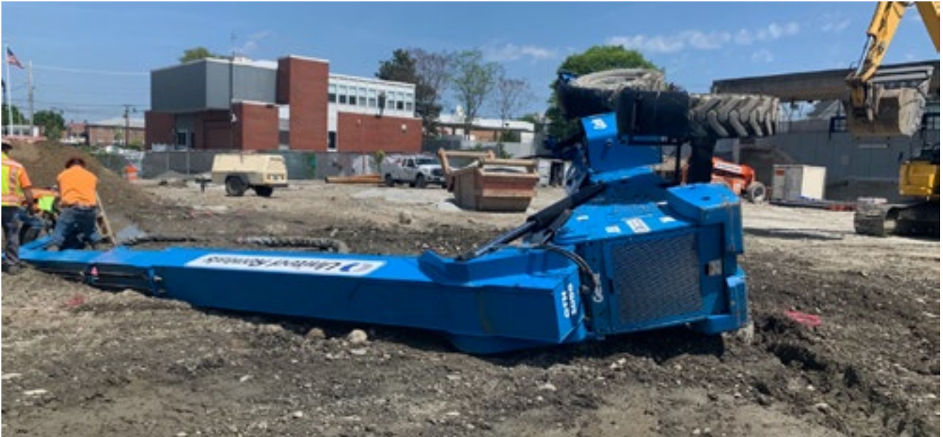
► A lull is tipped over after attempting to traverse an unstable Working Platform.
