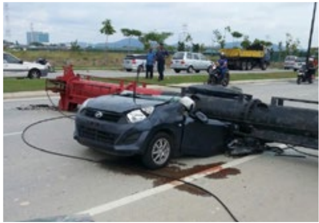
► Accident Involving a Piling Rig Image source: Guide to Working Platforms By the Joint EFC/DFI Working Platform Task Group 1st Edition December 2019
