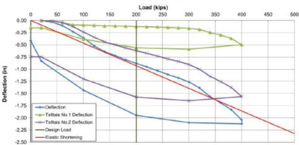
Friction Ductile Iron Pile - Compression Load Test Load vs. Deflection
