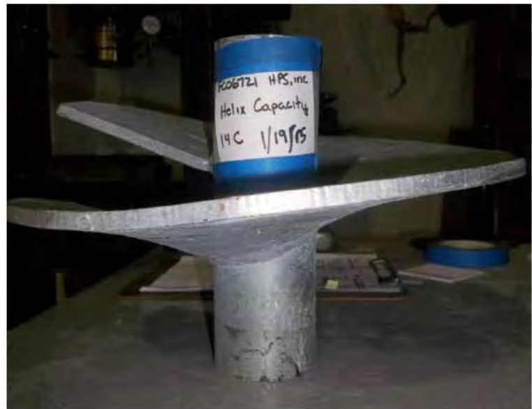
Fig. C-2 – RS2875 14" Dia. Helix – Test Results
